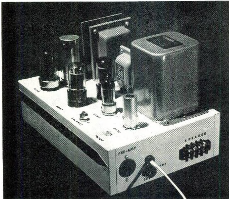
Fig. 1. External appearance of the authors' amplifier. Follow this layout for simplest wiring.
