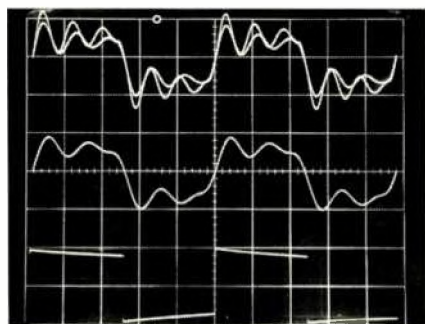
Fig. 4—Square-wave response of CAD-50SL in pentode mode at 10 kHz into 4-ohm and 8-ohm loads (overlaid traces, top), 10 kHz into 8 ohms paralleled by 2 \mu F (middle), and 40 Hz into 8 ohms (bottom). Scales: Vertical, 5 V/div.; horizontal, 20 \mu S/div. for 20-kHz traces, 5 ms/div. for 40-Hz trace.
