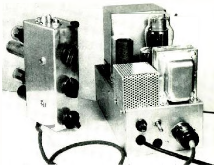
Fig. 1. Compact, two section amplifier with control section arranged for mounting in small panel area.
