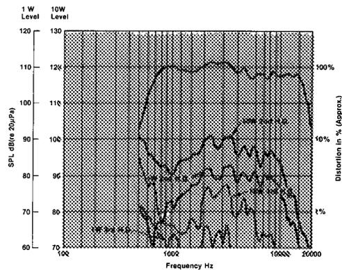
Second and third harmonic distortion curves of the 2370A with 1 watt (2.83 V RMS) and 10 watts (8.94 V RMS) applied to the JBL Model 2425H compression driver. Measured on axis at a distance of 1 meter in a reflection-free environment.
