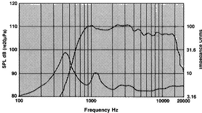
Frequency response of the 2370A, measured on axis at a distance of 1 meter with 1 watt (2.83 V RMS) applied to a JBL Model 2425H compression driver, in a reflection-free environment, with impedance vs frequency curve.
