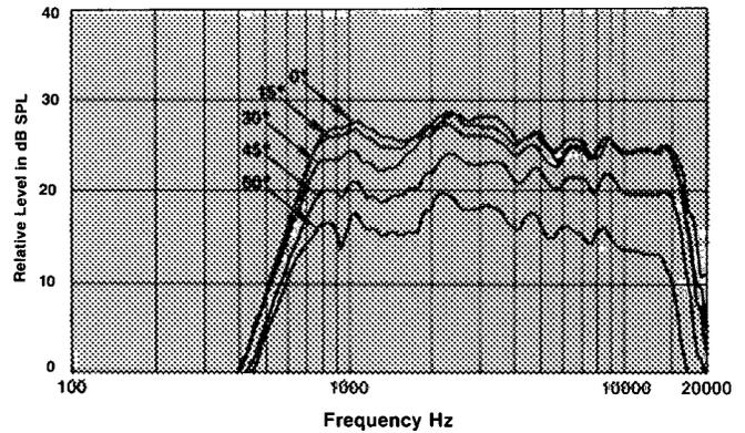
Horizontal off-axis response taken at 15 degree intervals out to 60 degrees off axis.
