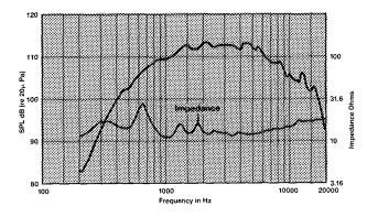
Frequency response of the 2450J coupled to a JBL 2380A Flat-Front Bi-Radial<sup>#</sup> Horn, measured on-axis at a distance of 1 meter with a l-watt (4.0 V RMS) input in a reflection-free environment, with impedance vs. frequency curve. A horn with a pure exponential flare, such as typical radial horn designs, will exhibit greater high frequency output on axis at the expense of lost annular coverage.
