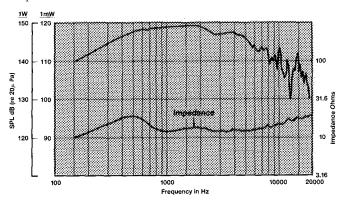
Frequency response and impedance modulus of Model 2450J coupled to a 49 mm (2 in) diameter terminated plane-wave tube, with sensitivity referenced to a 25 mm (1 in) tube. This is the power response of the transducer, and is the frequency response that will be obtained on a true full-range constant directivity horn design, such as JBL s 2360 series of Constant Coverage Bi-Radial<sup>\*</sup>Horns.
