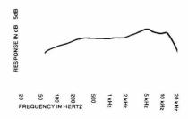
Created especially for TV, the small, lightweight 649B is the most popular dynamic lavalier available. The turned aluminum case and nested mechanical parts offer traditional E-V ruggedness. Frequency response is tailored for balanced performance in the lavalier chest position. The 649B is at home wherever concealment, mobility, and hands-free movement is needed.
