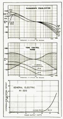
Fig. 1. Performance curves for the XA1-320 "convertible" amplifier.
