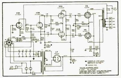
Fig. 4. Schematic of the power amplifier section.
