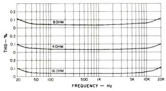
Fig. 2—THD versus frequency for 4-,8-, and 16-ohm loads at 50-watts output.
