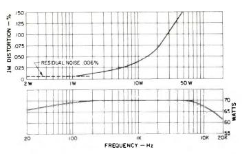
Fig. 3—The MB-3045's power characteristics. Top, SMPTE IM versus output, 8-ohm loads; Bottom, bandwidth for 1.0 per cent THD, 8-ohm loads.
