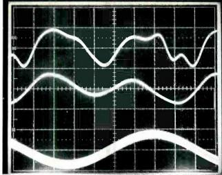
Fig. 4 — MB-3045's SMPTE IM residual at 50 watts, Top; and 15.8 watts, Center; with input at bottom.
