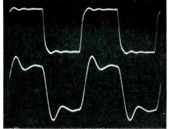
Fig. 6 — Response of the MB-3045 to a 10 kHz square wave into an 8 ohm load (Top), and into an 8 ohm load paralleled by 2 µF. Scale is 10V/div.
