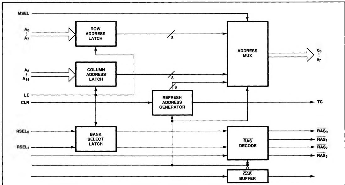
Figure 1. Block Diagram of 2964B Dynamic Memory Controller
