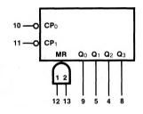
Vcc = Pin 14 GND = Pin 7 NC = Pins 1, 2, 3, 6
