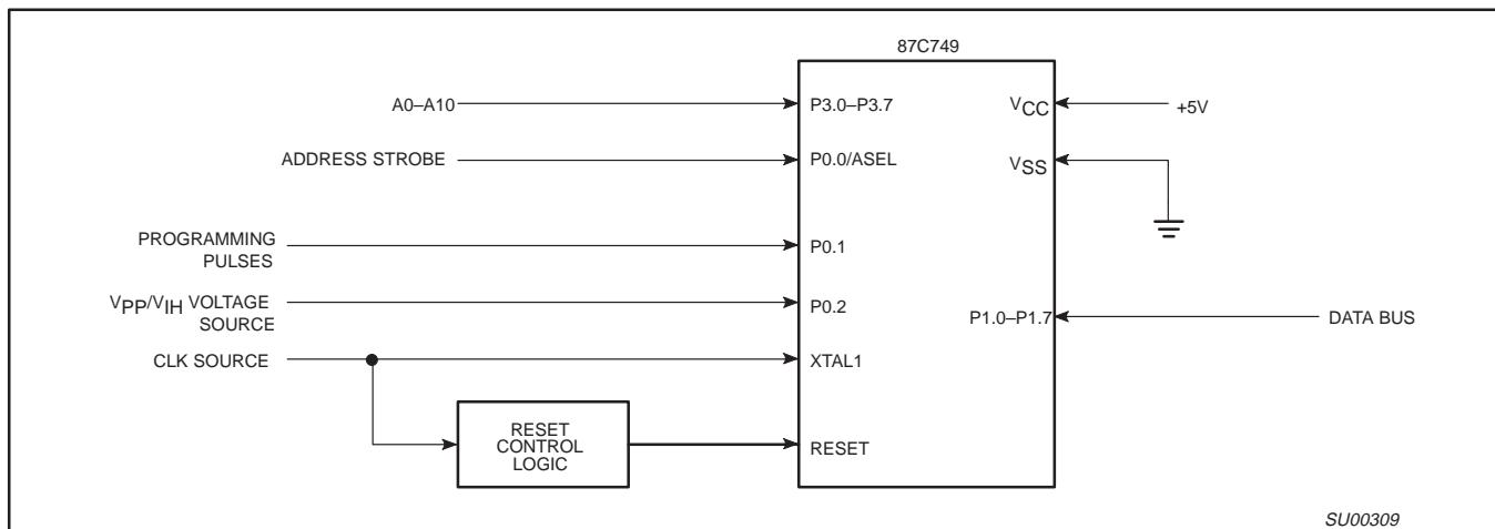
Figure 7. Programming Configuration
