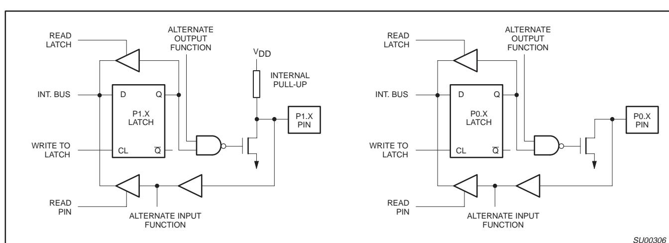
Figure 1. Port Bit Latches and I/O Buffers
