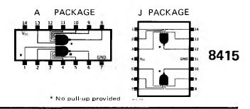
The 8415 is a Dual 5-Input NAND Gate with bare output collectors. Absence of an output pull-up structure allows the user complete freedom in the use of the 8415 in collector-logic (wired-AND) and similar applications. Proper pull-up resistor selection will allow as many as 30 outputs to be tied together.
