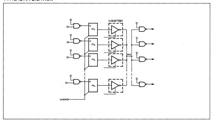
The above figure illustrates usage of the 8T09 in data processing logic. For example,  $FF_1$  thru  $FF_n$  may represent bit X in each of several functions in a minicomputer (accumulators, MQ register, index registers, indirect address
