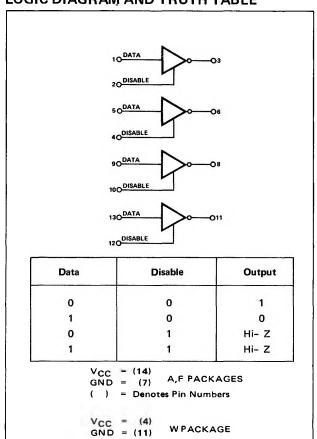
(control input "0"). This eliminates the resistor pull-up requirement while providing performance superior to open collector schemes. Each output can sink 40mA and drive 300pF loading with guaranteed propagation delay less than 22 nanoseconds.
