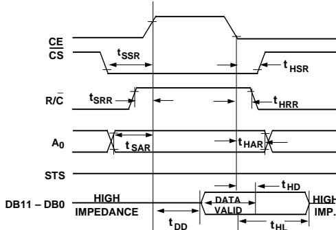
Figure 2. Read Cycle Timing
