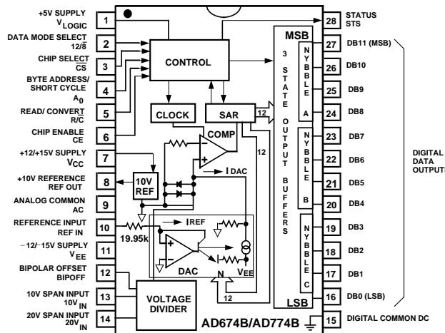
Figure 5. Block Diagram of AD674B and AD774B
