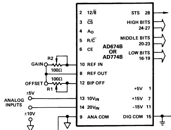
*Figure 8. Bipolar Input Connections*
