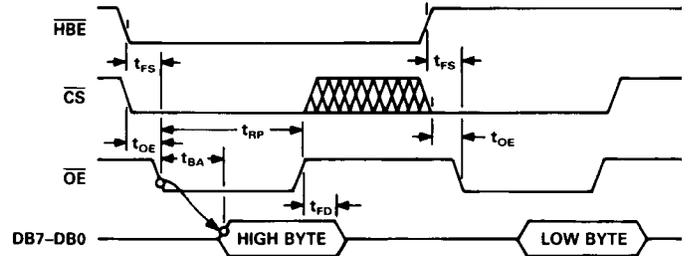
Figure 2. Output Timing
