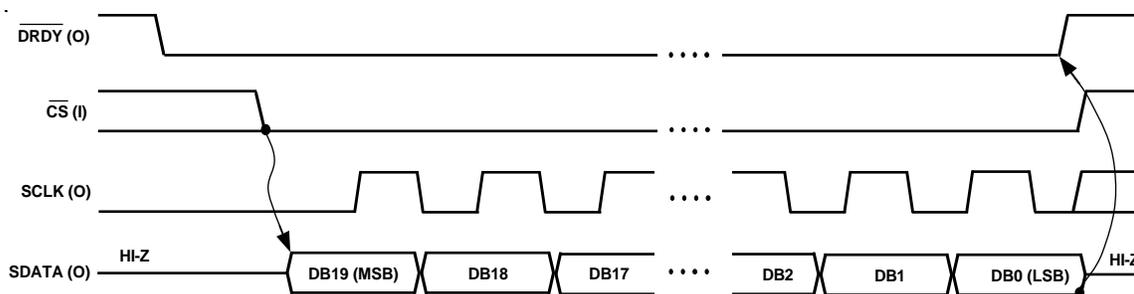
Figure 17. Timing Diagram for the SEC Mode
