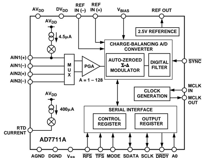
CMOS construction ensures low power dissipation, and a software programmable power-down mode reduces the standby power consumption to only 7 mW typical. The part is available in a 24-lead, 0.3 inch-wide, hermetic dual-in-line package (cerdip) as well as a 24-lead small outline (SOIC) package.
