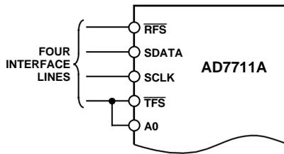
Figure 14. Simplified Interface with  $\overline{\text{TFS}}$  Connected to A0
