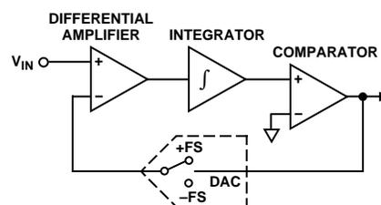
Figure 5. Basic Charge-Balancing ADC
