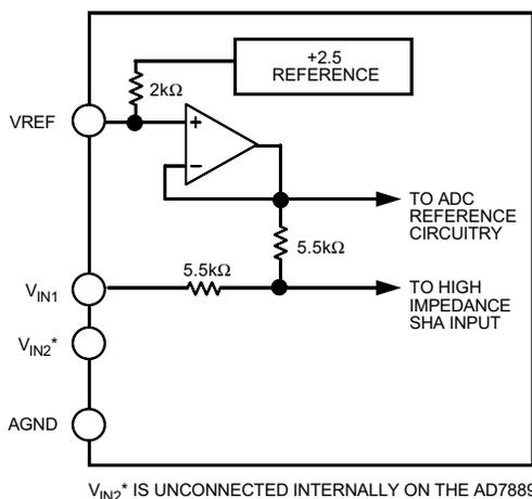
*Figure 5. AD7889-3 Analog Input Structure*
