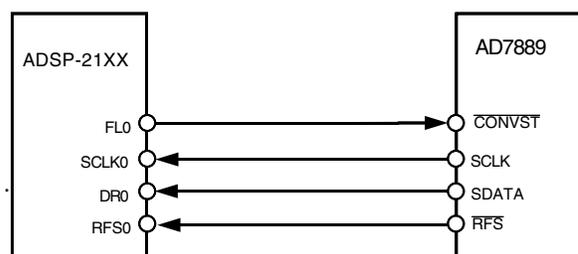
*Figure 6. AD7889 to ADSP-21XX Interface*
