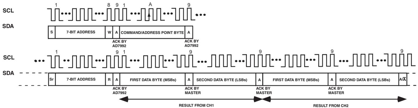
Figure 18. Mode 2 Sequence Operation
