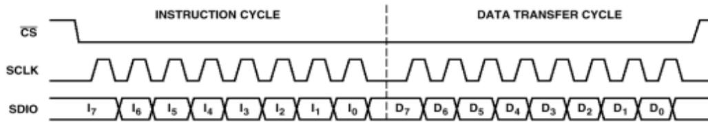
Figure 34. Serial Port Writing Timing—Clock Stall Low
