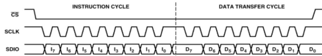
Figure 36. Serial Port Write Timing—Clock Stall High
