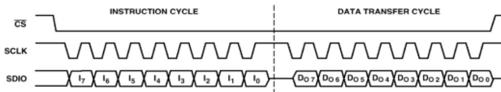
Figure 37. Two-Wire Serial Port Read Timing—Clock Stall High
