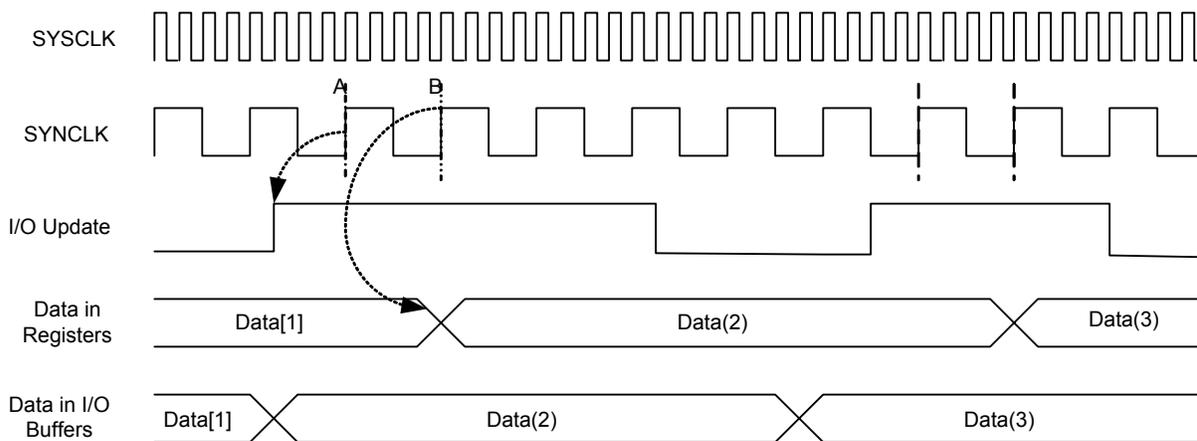
The device registers an I/O Update at point A. The data is transferred from the asynchronously loaded I/O buffers at point B.
