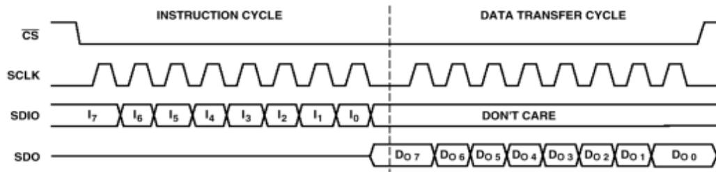
Figure 35. Three-Wire Serial Port Read Timing—Clock Stall Low
