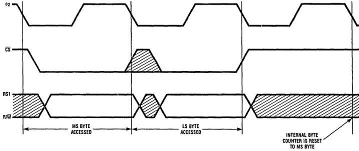
Timing for a Typical  $\mu$ P 8 Byte Access
