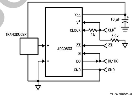
**FIGURE 7. Remote Sensing—Clock and Power on 1 Wire**
