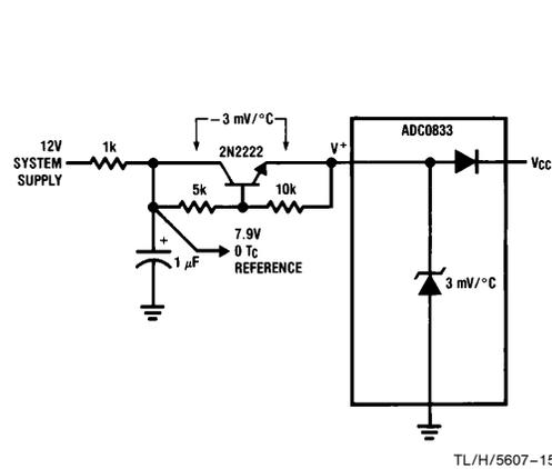
**FIGURE 4. Operating with a Temperature Compensated Reference**
