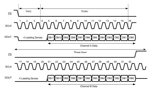
Figure 1. ADC122S655 Single Conversion Timing Diagram
