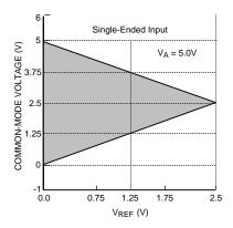
Figure 37. V<sub>CM</sub> range for single-ended operation
