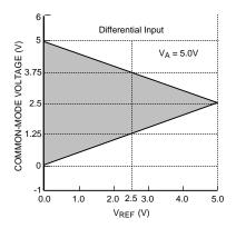
Figure 36. V<sub>CM</sub> range for Differential Input operation
