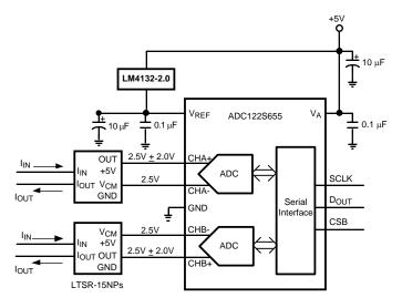
Figure 39. Interfacing the ADC122S655 to a Current Transducer
