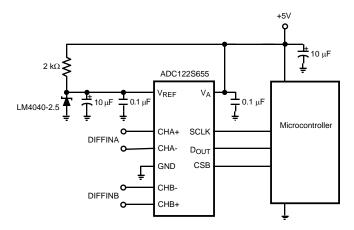
Figure 38. Low cost, low power Data Acquisition System
