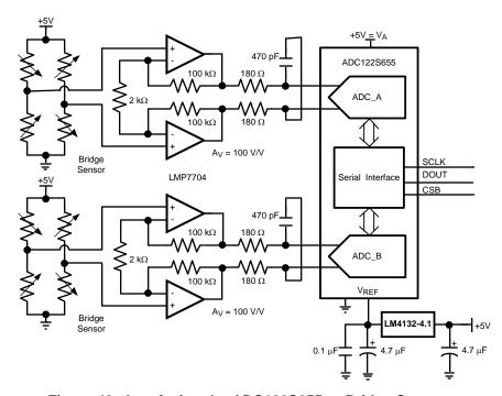
Figure 40. Interfacing the ADC122S655 to Bridge Sensors
