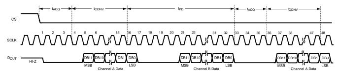
Figure 2. ADC122S655 Continuous Conversion Timing Diagram
