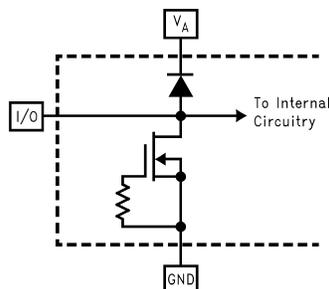
Figure 1. ESD Protection Scheme for Digital Input pins
