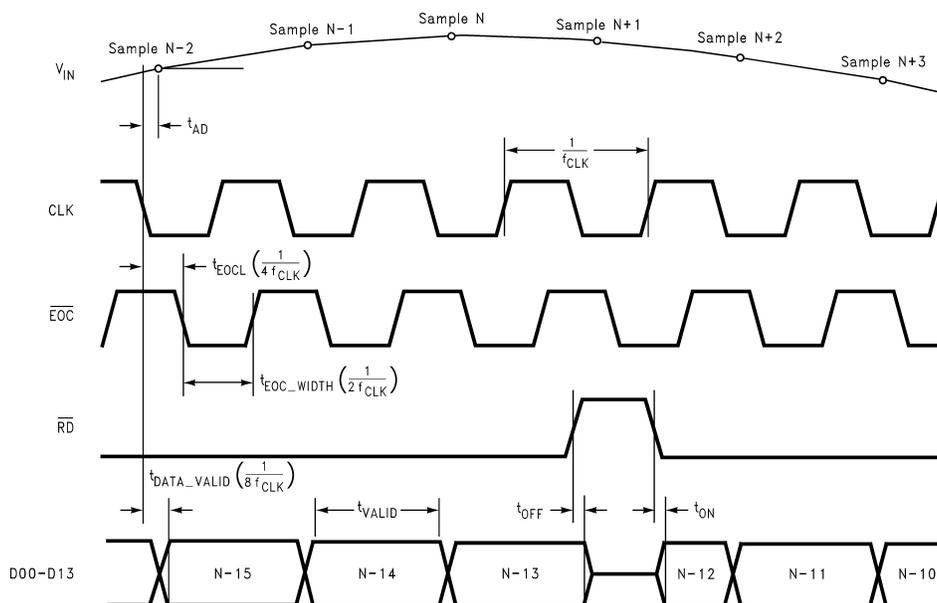
**Figure 3. TIMING DIAGRAM 1. Output Timing**
