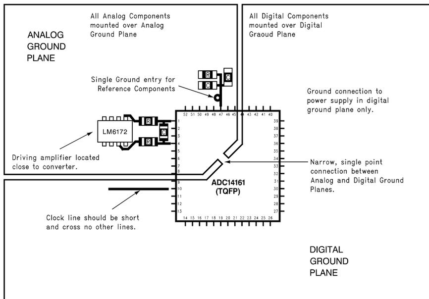
Figure 11. Example of a suitable layout.
