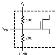
**Figure 7.  $V_{CM}$  input to the ADC14161  $V_{CM}$  is set to 40% of  $V_A$  with on-chip resistors. Performance is improved when  $V_{CM}$  is driven with a stable, low impedance source**
