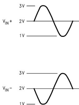
**Figure 6. Expected Input Signal Range.**
