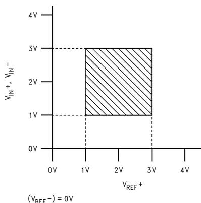
**Figure 5. Typical Input to Reference Relationship.**
