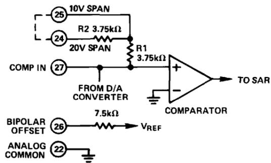
Figure 11. AD ADC71/AD ADC72 Input Scaling Circuit
