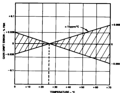
Figure 3. AD ADC71 Gain Drift Error vs. Temperature
