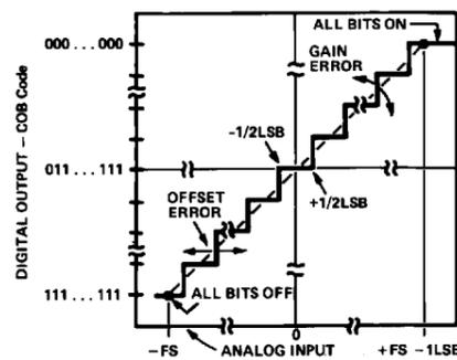
Figure 4. Transfer Characteristics for an Ideal Bipolar A/D
