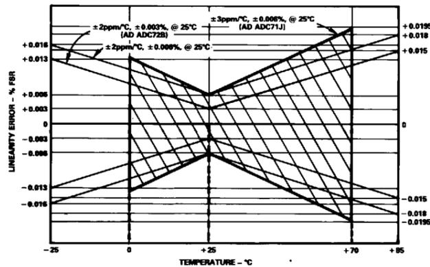
Figure 1. Linearity Error vs. Temperature
