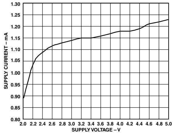
TPC 11. Supply Current vs. Supply Voltage
