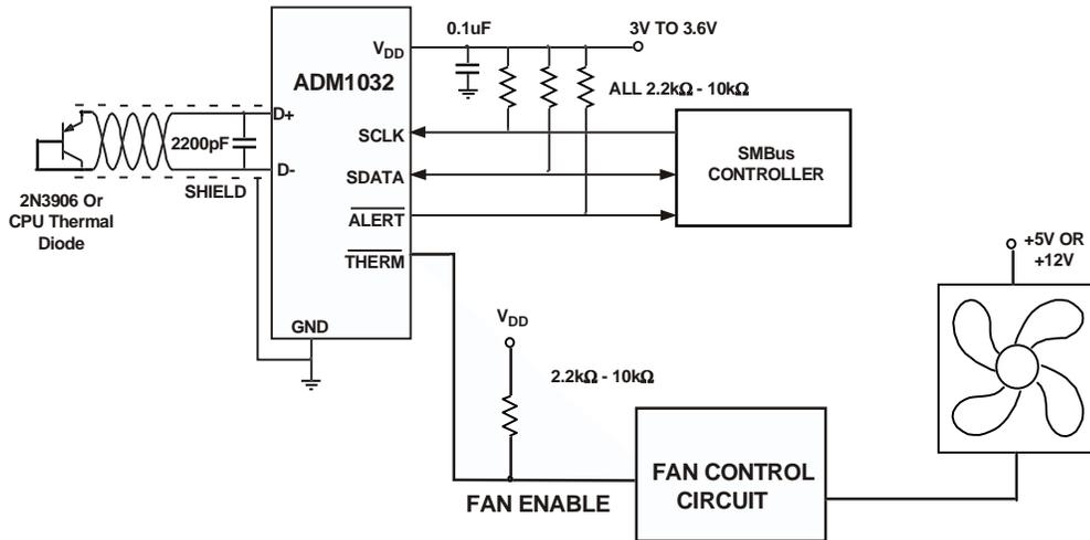
Figure 14. Typical ADM1032 Application Circuit
