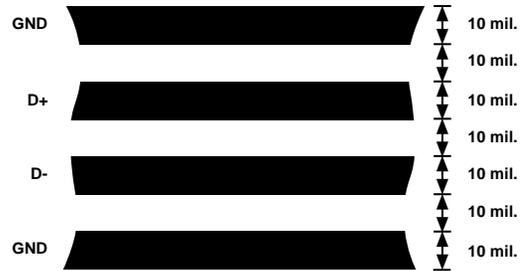
Figure 5. Arrangement of Signal Tracks
