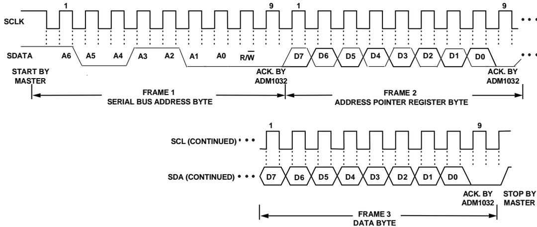
Figure 3a. Writing a Register Address to the Address Pointer Register, then Writing Data to the Selected Register
