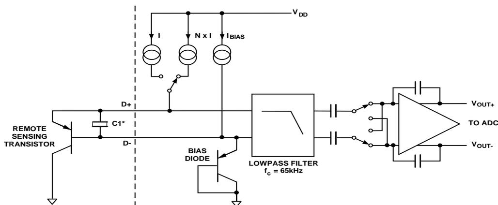
\*Capacitor C1 is optional. It is only necessary in noisy environments.
