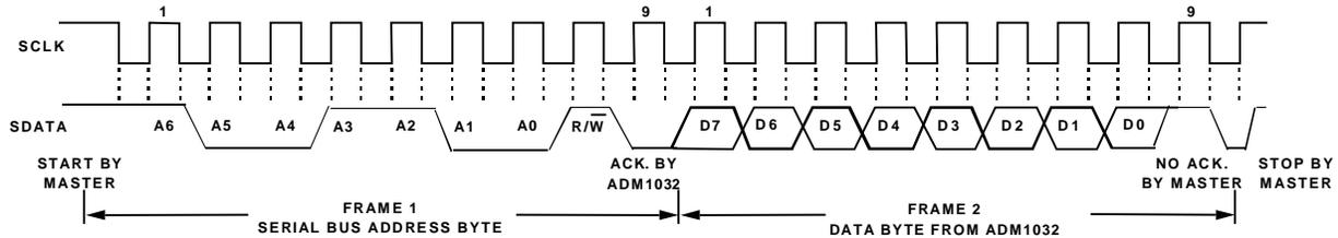
Figure 3c. Reading Data from a Previously Selected Register
