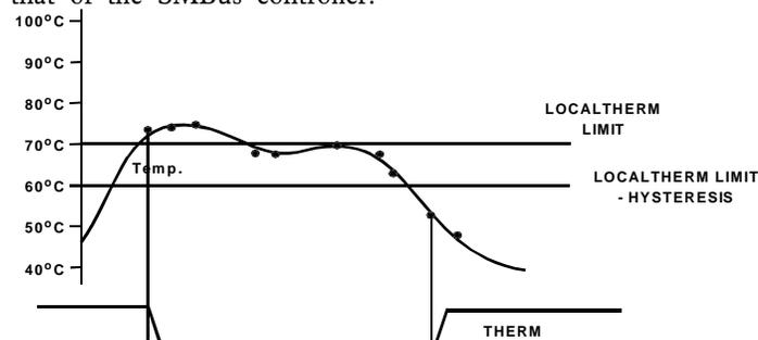
Figure 13. Operation of the  $\overline{\text{THERM}}$  Output
