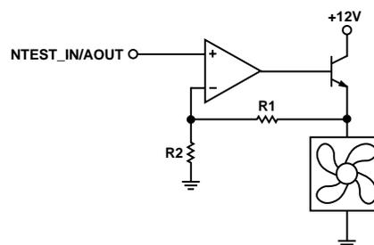
Figure 5. Analog Output Driving Fan
