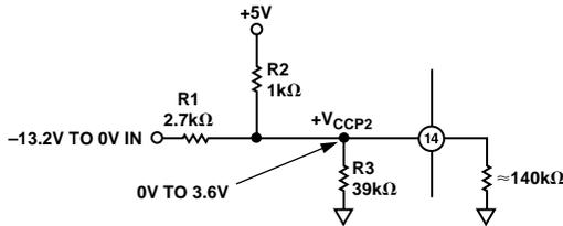
Figure 4. Scaling  $V_{CCP2}$  to  $-12\text{ V}$  ( $+10\%$ )
