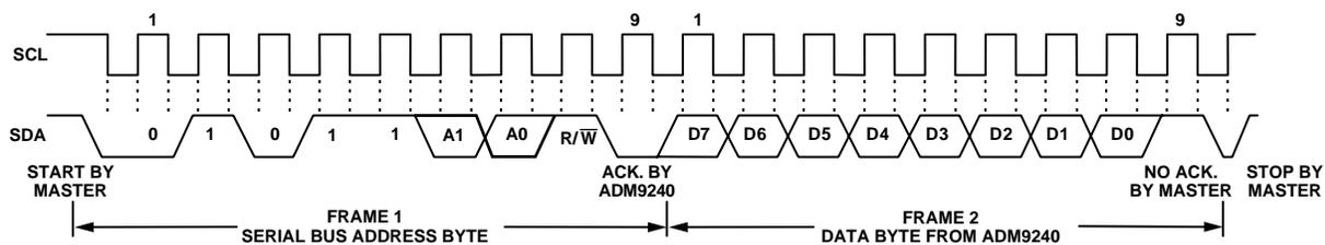
Figure 2c. Reading Data from a Previously Selected Register
