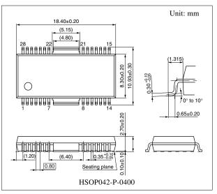
Note) The package of this product will be changed to lead-free type (HSOP042-P-0400D). See the new package dimensions section later of this datasheet.
