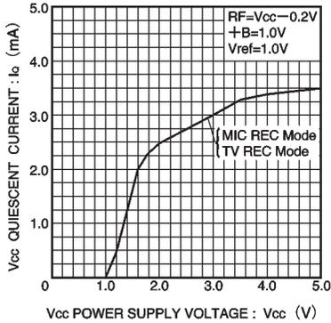
Fig. 3 Vcc quiescent current vs. power supply voltage
