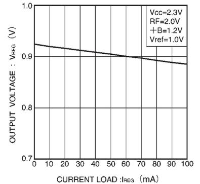
Fig. 17 Regulator output voltage vs. load current
