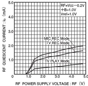
Fig. 4 RF quiescent current vs. power supply voltage
