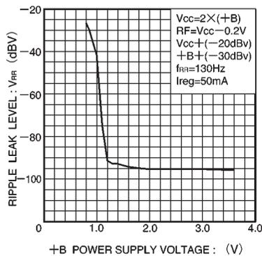
Fig. 18 Regulator ripple leak vs. power supply voltage
