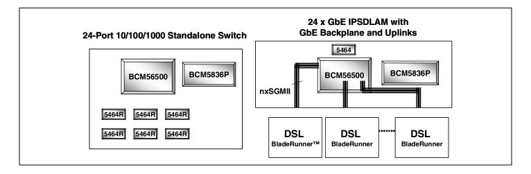
The BCM56500 is the fifth generation of the highly-integrated and cost-effective StrataSwitch and StrataXGS product line in a single-chip solution with 24-GbE ports. The BCM56500 incorporates 24-GbE ports that can operate 10/100/1000 Mbps.
