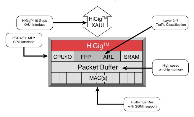
The **BCM5690** network switch is a scalable, modular chip solution with 12 ports. Each of these flexible ports supports Gigabit Ethernet or 10/100 Mbps Ethernet. Additionally, the **BCM5690** supports both copper and fiber physical interfaces. The **BCM5690** has a fully integrated SerDes functionality consisting of a 10 Gbps XAUI HiGig Port, Gigabit Ethernet or a SGMII PHY interface.
