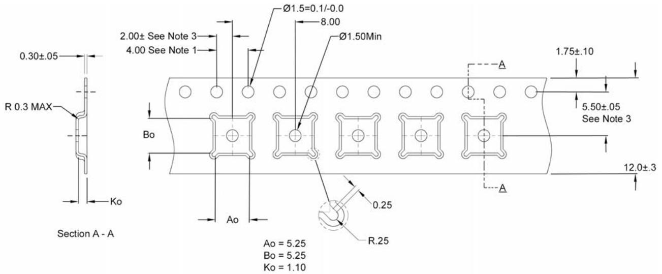
**Figure 14. CABGA Carrier Tape Drawing**
