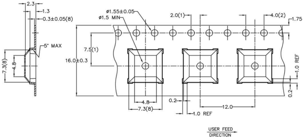
1. Measured from the centerline of sprocket hole to centerline of the pocket hole and from the centerline of sprocket hole to centerline of the pocket.
