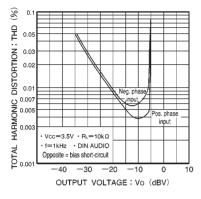
Fig. 3 Output voltage vs.distortion
