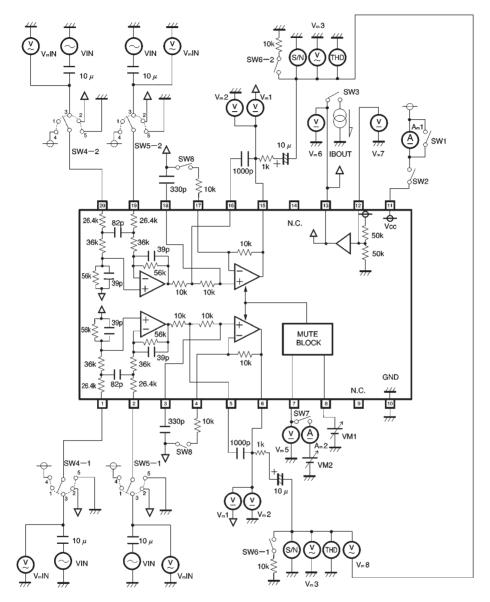
Note 1: Arrows indicate the positive current direction. Note 2: Unless otherwise noted, AC input (VIN) = 1 kHz sine waves. Note 3: Unless otherwise noted, SW8 = Off.
