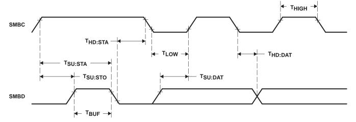
Figure 1. SMBus Timing Data
