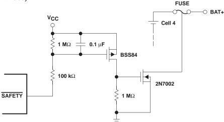
Figure 7. Example SAFETY Circuit Implementation
