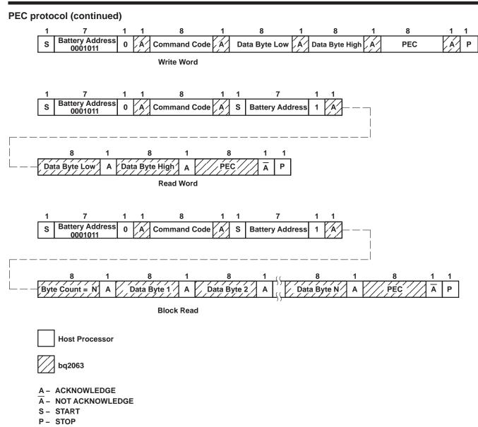
Figure 9. SMBus Communication Protocol With PEC
