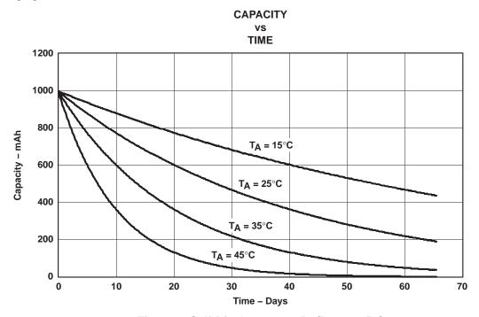
Figure 6. Self-Discharge at 2.5%/Day at 25°C
