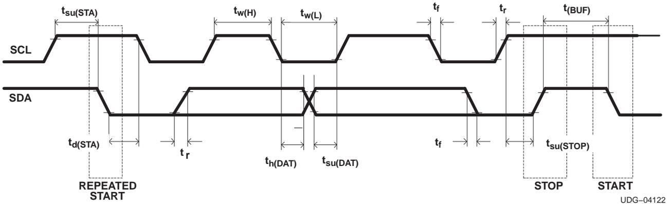
Figure 2. I<sup>2</sup>C Timing Diagram
