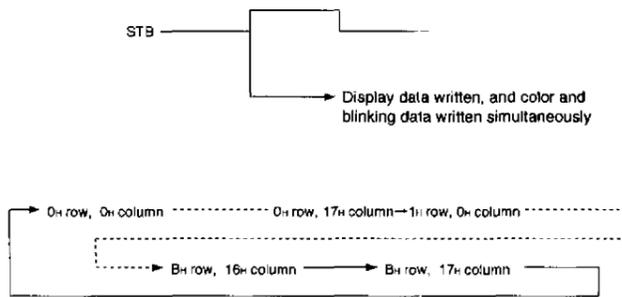
\* 1)The address counter is incremented after the RAM data is written. It is not effected by the STB pulse width.
