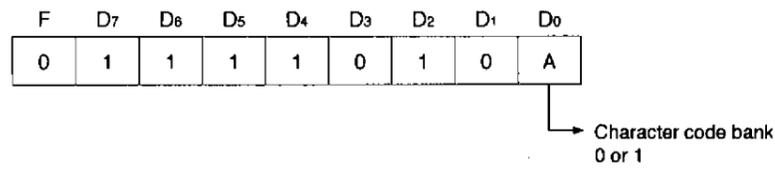
With the BU2870FS, use 0 and 1 to select between the two banks of 128 characters. This command does not apply to the BU2848FS and BU2873FS.
