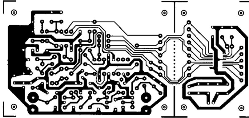
●PCB for application example circuit (component side)
