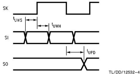
**FIGURE 3. MICROWIRE/PLUS Timing**
