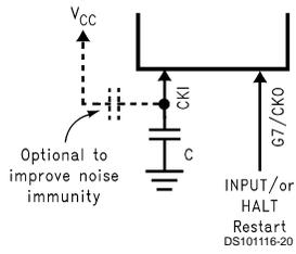
For operation at lower than maximum R/C oscillator frequency.
