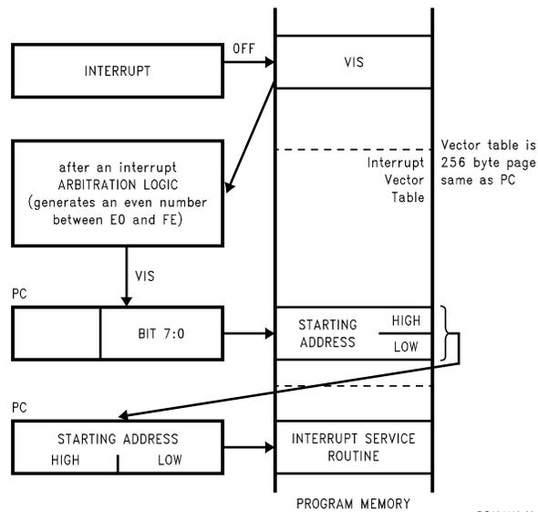
FIGURE 27. VIS Operation
