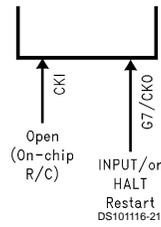
For operation at maximum R/C oscillator frequency.
