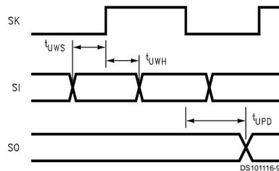
**FIGURE 4. MICROWIRE/PLUS Timing**
