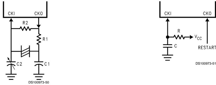
FIGURE 10. Crystal and R/C Oscillator
