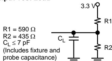
(b) CML Output Test Load<sup>[27]</sup>
