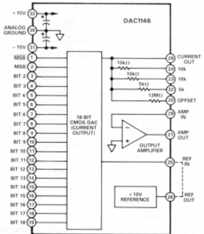
Figure 1. DAC1146 Block Diagram
