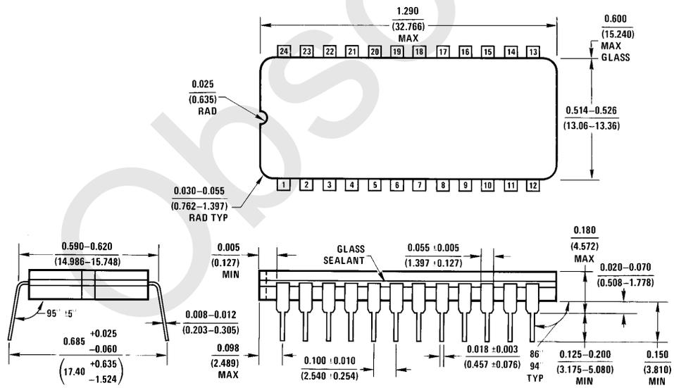
**24-Lead Ceramic Dual-In-Line Package (J)**
