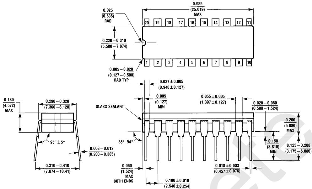
**20-Lead Ceramic Dual-In-Line Package (J)**
