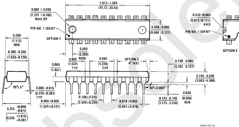
**20-Lead Molded Dual-In-Line Package (N)**
