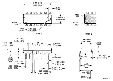
14-Lead Molded Dual-In-Line Package (N) Order Number DM7406N Package Number N14A
