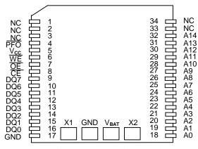
34-Pin PowerCap Module Board (Uses DS9034PCX PowerCap)
