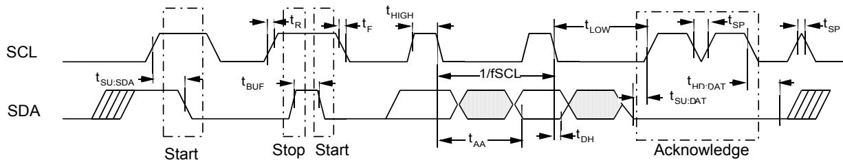
**Write Bus Timing**
