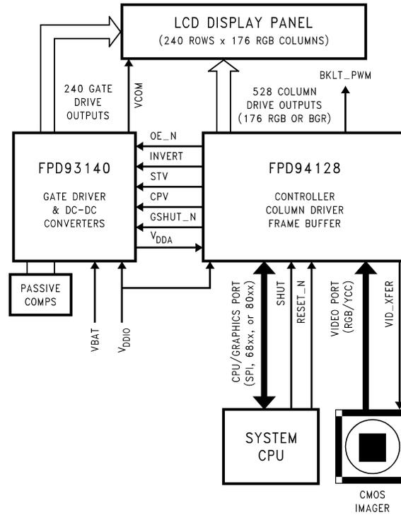
Figure 2. FPD94128 Block Diagram
