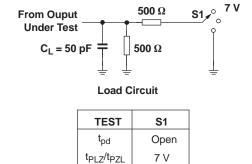
$\begin{tabular}{l|l} $t_{PHZ}/t_{PZH}$ & Open \\ \hline \\ $C_L = Load$ capacitance, includes jig and probe capacitance (see $AC$ Characteristics for value). \\ \hline \end{tabular}$
