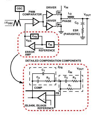
FIGURE 6. VOLTAGE-MODE BUCK CONVERTER COMPENSATION DESIGN
