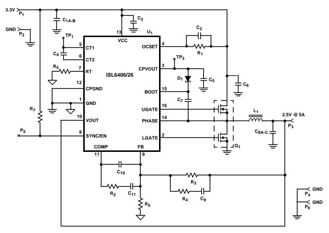
NOTE: Remove R3, R4, C9, and R5 from the board for ISL6426 evaluation.
