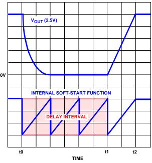
FIGURE 4. OVERCURRENT PROTECTION RESPONSE
