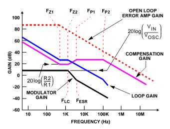
FIGURE 7. ASYMPTOTIC BODE PLOT OF CONVERTER GAIN
