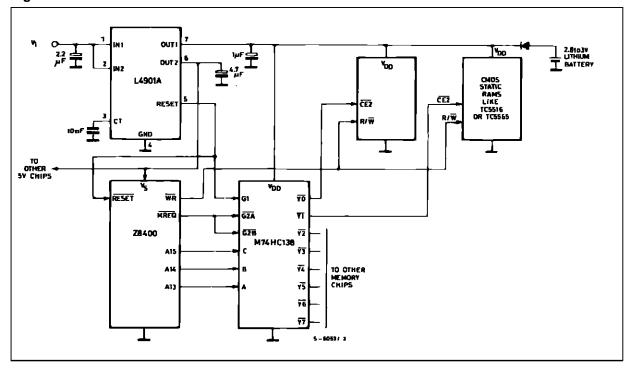
Another interesting application of the L4901A is in  $\mu P$  system with shadow memories (see Figure 6). When the input voltage goes below  $V_{IT}$ , the reset ouput enables the execution of a routine that saves the machine's state in the shadow RAM (xicor x 2201 for example).
