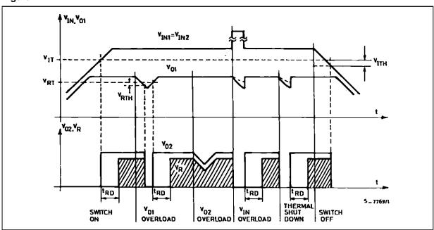
This output may therefore be used to supply circuits continuously, such as volatile RAMs, allowing the use of a back-up battery. The  $V_{01}$  regulator also features low consumption (0.6 mA typ.) to minimize battery drain in applications where the  $V_1$  regulator is permanently connected to a battery supply.
